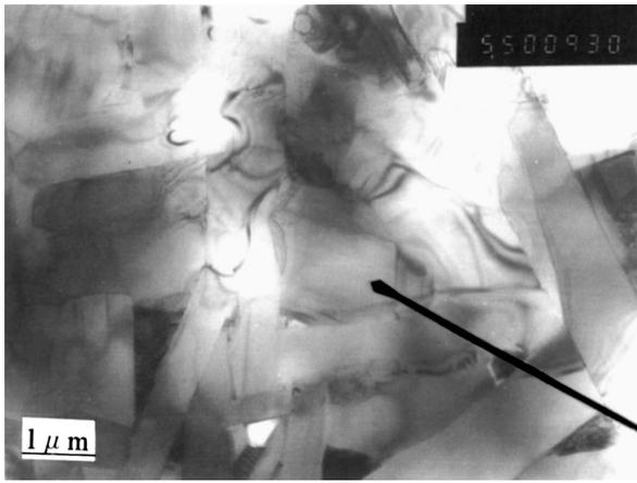
Figure 3 The fracture surface of SiC-AlN showing rods structure.
