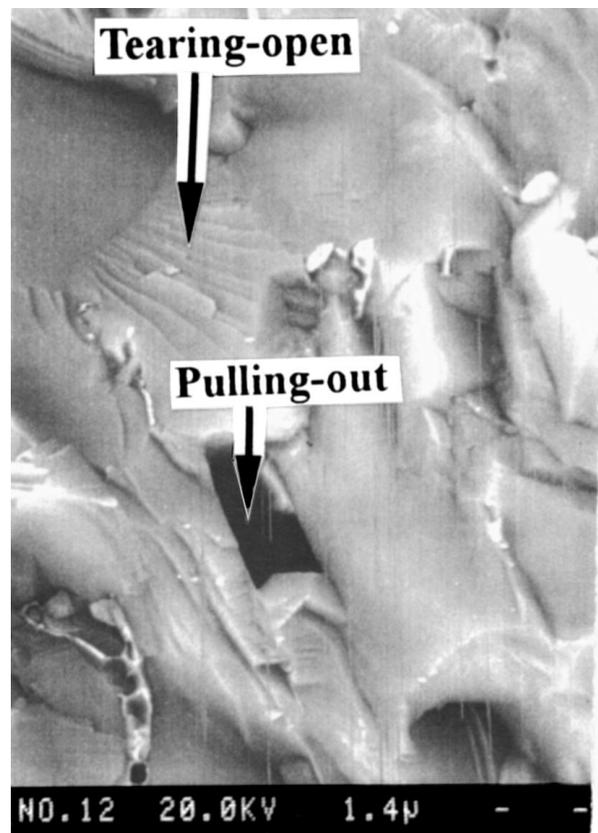
Figure 2 The fracture of SiC–AlN pulling-out and tearing-open phenomenon.
