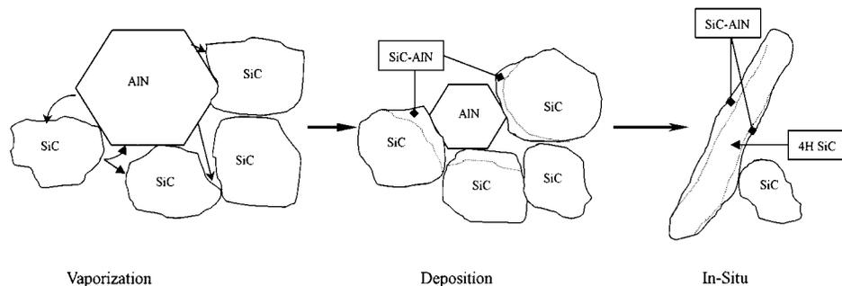
Figure 6 The schematic for in-situ characterization of SiC–AlN multiphase ceramics.
