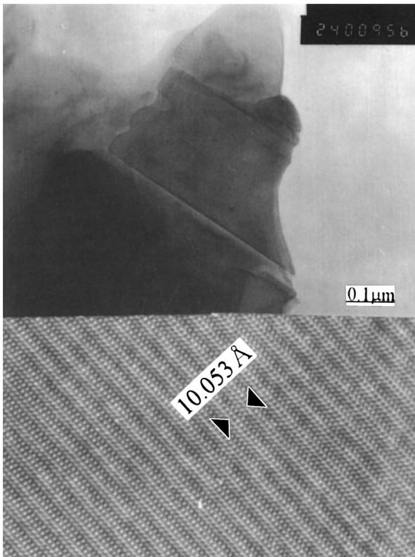
Figure 4 The 4H phase of SiC rod crystal core by TEM.
